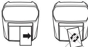
**!** If a banknote is placed into the loading tray incorrectly, it will not be identified as genuine, and an error code will be displayed.
