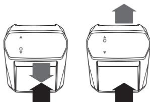
**!** We recommend using the Forward mode for a bundle of banknotes. The Backward mode is convenient in case of limited space (e.g. when the detector is placed against the wall) or to verify a single banknote.
